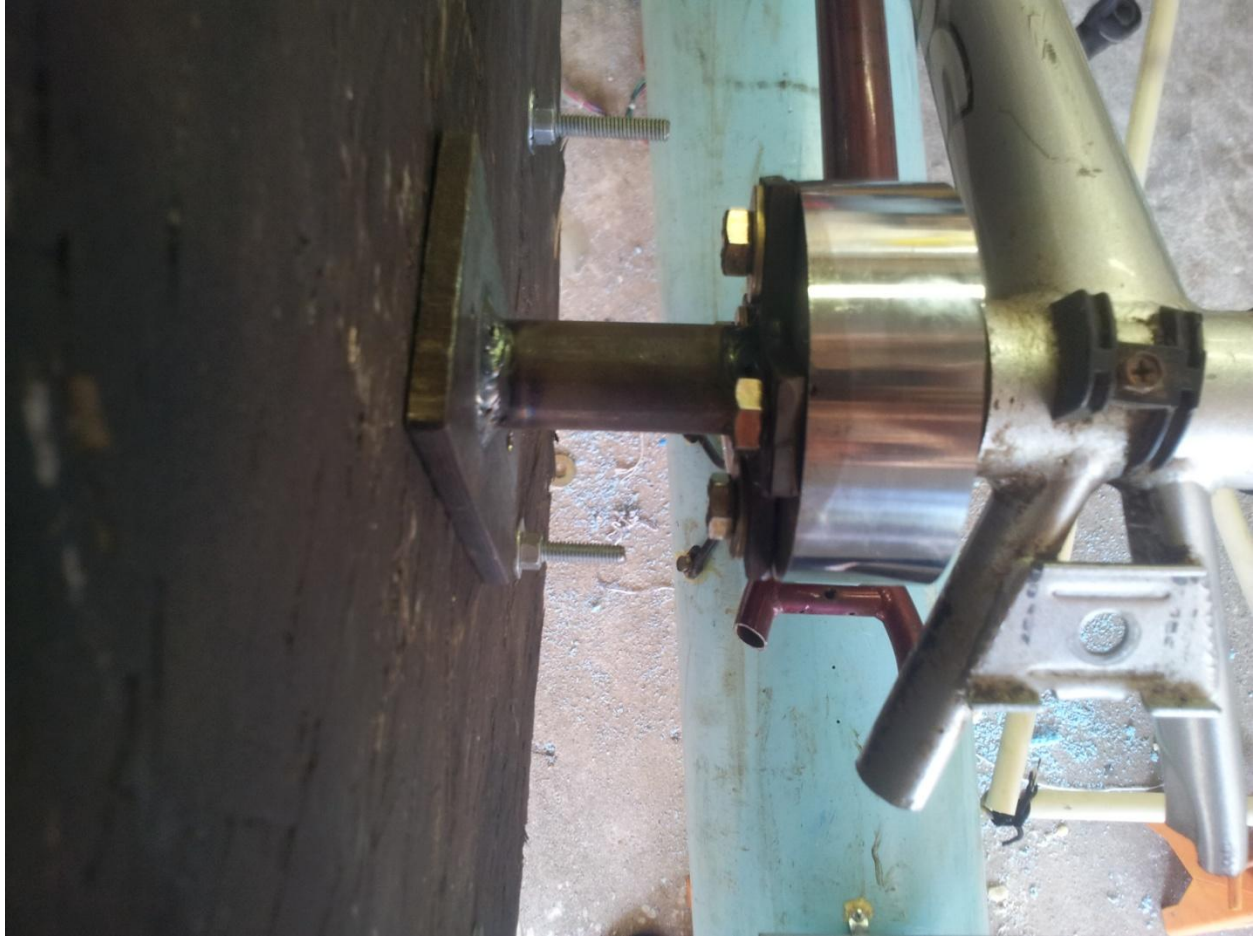
Figure 36 – Machined Steel Rod and Plate Supporting Paddle Wheel
