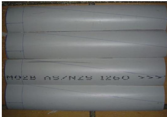
Figure 17 – Sample PVC cuts to approximate airfoil shape. "YourGreenDream"
