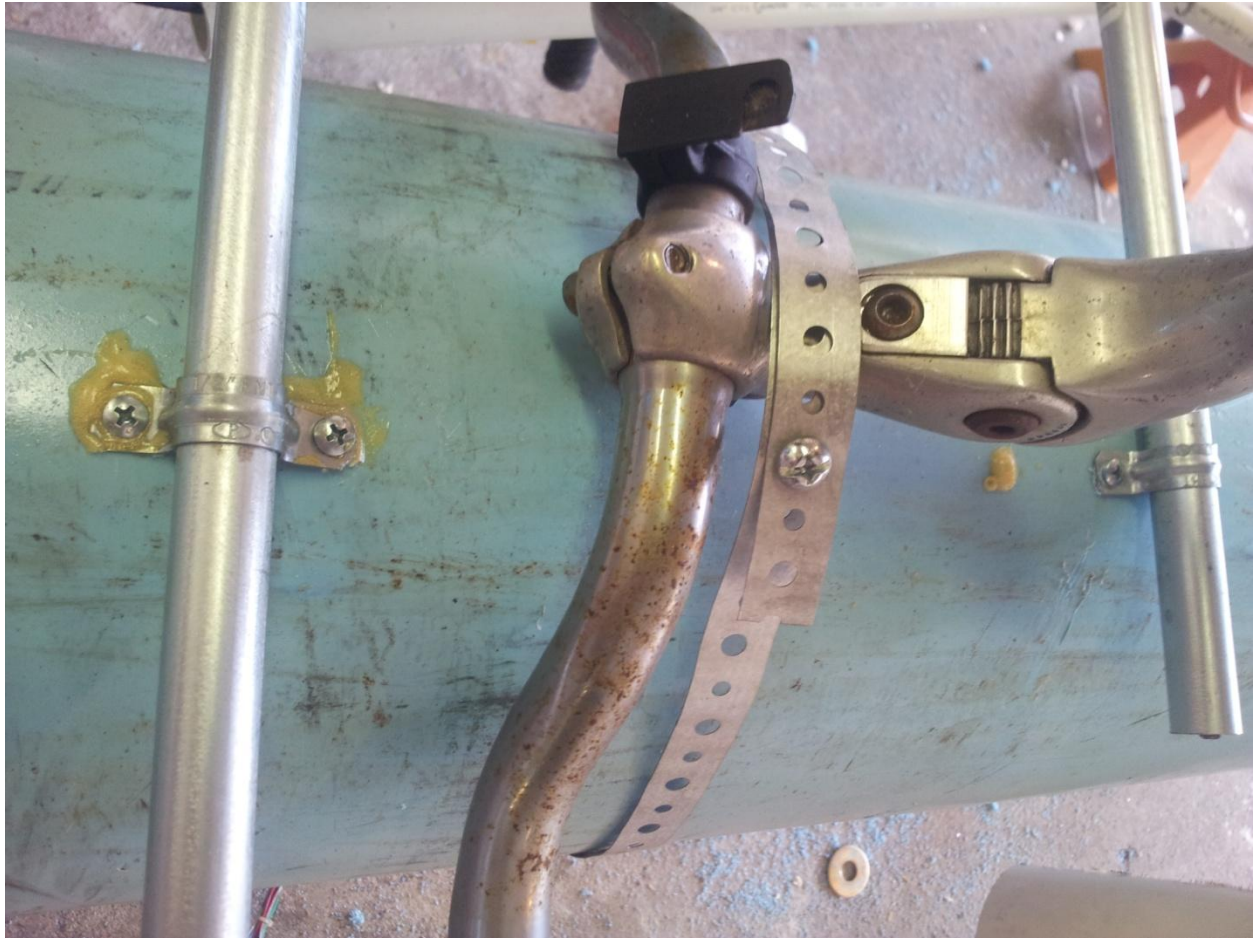
Figure 39– Straps Holding Handlebars of MHET against Floating PVC
