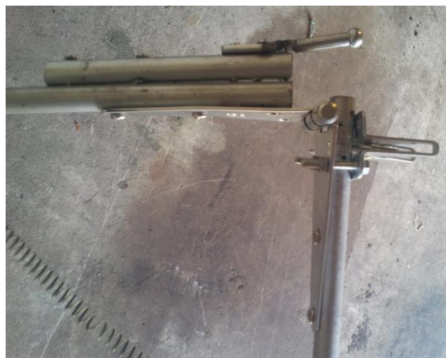
Figure 28 – Break-away mechanism in triggered position
