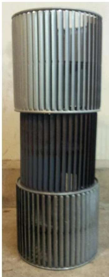
Figure 15 – Blower Fan Assemblies.
