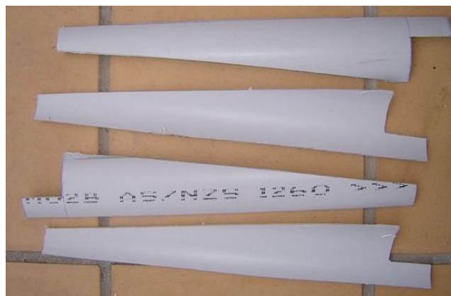
Figure 18 – Sample PVC cuts to approximate airfoil shape. "YourGreenDream"
