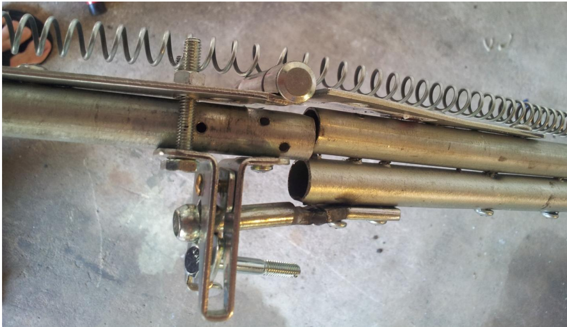
Figure 27 – Break-away mechanism in cocked position
