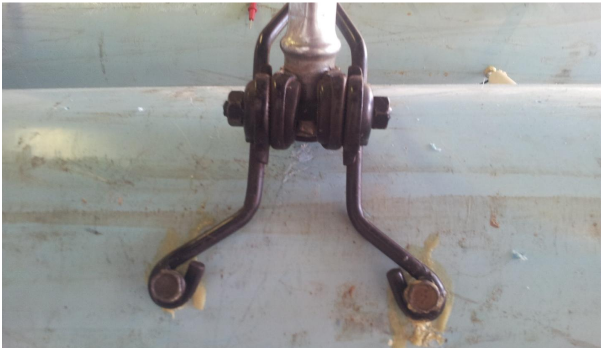
Figure 38 – Bicycle Seat Held to Floating PVC
