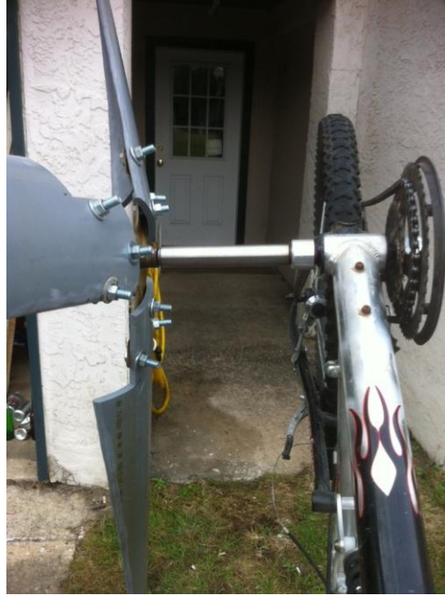
Figure 24 – Energy transfer axis on HAWT
