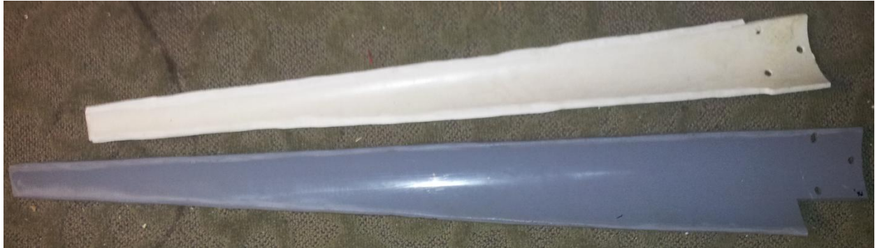
Figure 26 – Example of both 8-in (gray) and 6-in (white) diameter HAWT blades.
